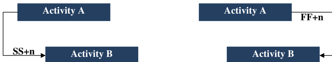
Figure 4-3: Starting successor activity n days after starting predecessor activity (left), and finishing successor activity n days after finishing predecessor activity (right)
